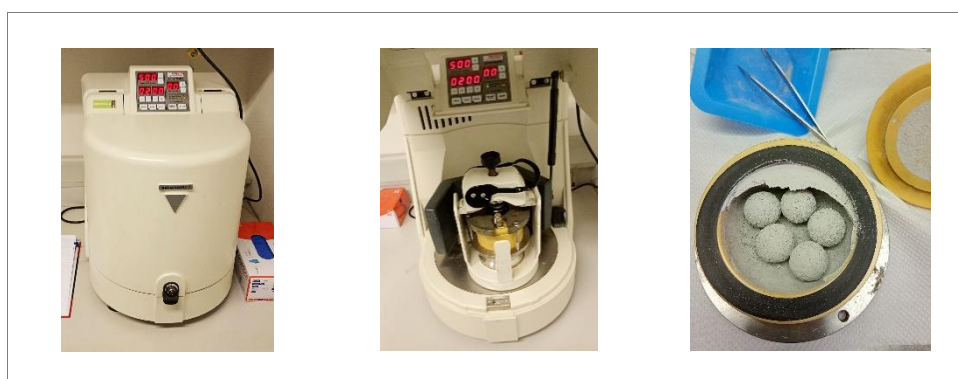
Figure 1: Photos of the Fritsch Planetary Mono Mill Pulverisette 6 (FRITSCH GmbH, Idar-Oberstein, Germany) used for glacial crushing experiments. From left to right: closed ball mill, open ball mill with the yellow grinding bowl, open grinding bowl after the crushing. Photos by Klara Köhler
